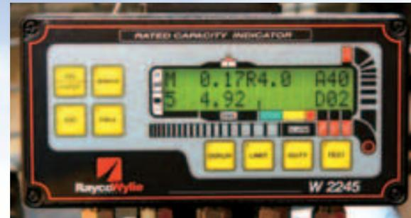
To prevent over-turning of the crane due to overload, sounds buzzer and stops crane operation automatically (hook hoisting, boom lowering and boom extending) when reaching the limit. Indicates digitally the rated load, actual load, working radius, boom length and boom angle. Operator settable limits.
