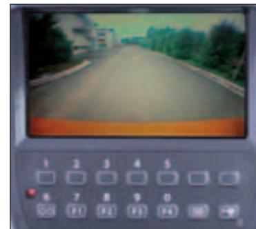
The widescreen color LCD, teamed up with the rear view camera on the counterweight provides rearward viewing.
